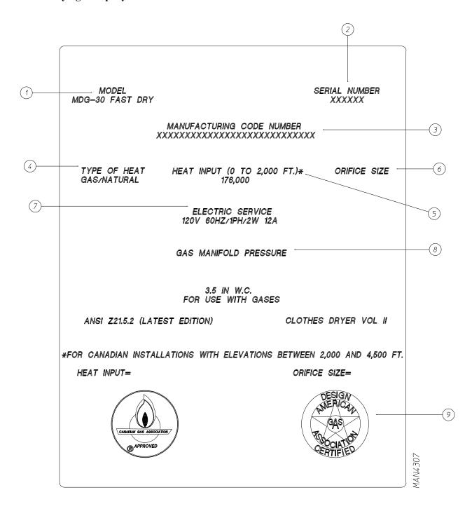
When contacting the **Maytag Co.** certain information is required to ensure proper service and parts information from the manufacturer. This information is on the data label located on the inside of the control door. When contacting the **Maytag Co.** please have the <u>model</u> and <u>serial numbers</u> available.
